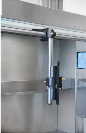
Camera holder mounted to the railing system KA-H-400 Art. No. 060.015.085
