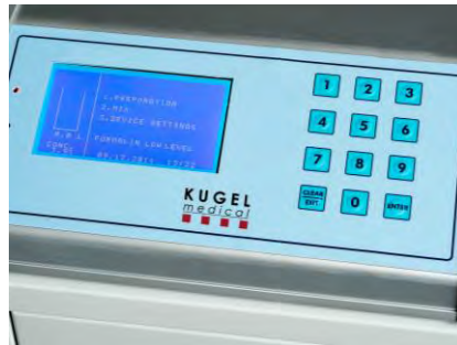
The fully automatic formalin mixing and dispensing station AFMDS-100 is designed for contact-free dilution of concentrated formalin in laboratories. Thanks to its compact design, the mixing station is also suitable for small laboratories. The integrated microprocessor within the device allows you to easily control all operations, such as mixing a 3.7% standard solution, through one single surface at the control panel with LCD display. Additionally, it is possible to prepare a customized mixture by using variable quantities of formalin, purified water and a buffer liquid. The prepared mixture can be drained directly from a tap at the device or transferred to multiple remote stations that are up to 200 meters away. Art. Nr. 099.900.196
